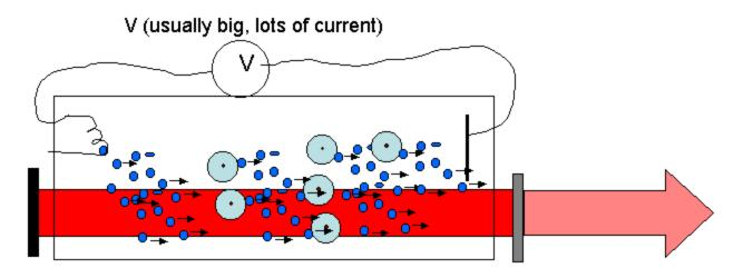
gas laser like Helium Neon. Just like neon sign with helium and neon mixture in it and mirrors on end.
