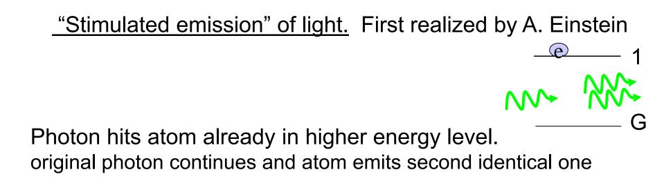
second identical photon comes out. Atom jumps down. Cloning photon. How to produce laser light?
