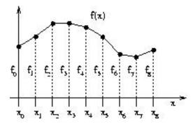
Notice, though, that there is one slope for every interval  $(x_i, x_{i+1})$  so the vector containing the slopes has one fewer entry than the vector F. The formula for the slope in the interval  $(x_i, x_{i+1})$  is  $(f_{i+1} - f_i)/h = N(f_{i+1} - f_i)$  where h = 1/N is the distance  $x_{i+1} - x_i$ . Thus the vector containing the slopes is
