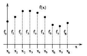
If this is all we have to work with, what should be use as an approximation to f'(x)? It seems reasonable to use the slopes of the line segments joining our sampled points.
