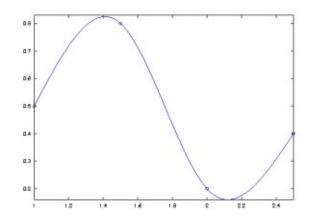
I have automated the procedure above and put the result in two files splinemat.m and plotspline.m. splinemat(n) returns the  $(n-1) \times (n-1)$  matrix used to compute a spline through n points while plotspline(X,Y) plots the cubic spline going through the points in Y and Y If you put these files in you MATLAB/Octave directory you can use them like this:
