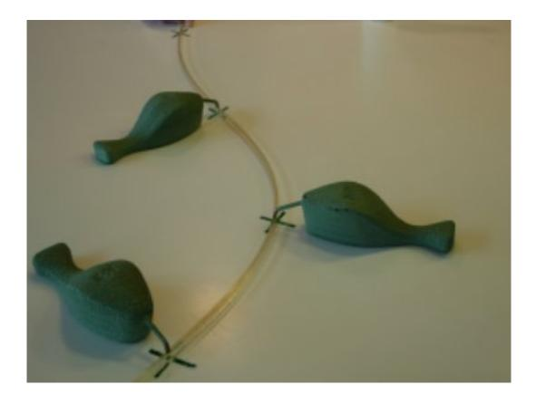
It consists of a bendable but stiff strip held in position by a series of weights called ducks. We will try to make a mathematical model of such a device.
